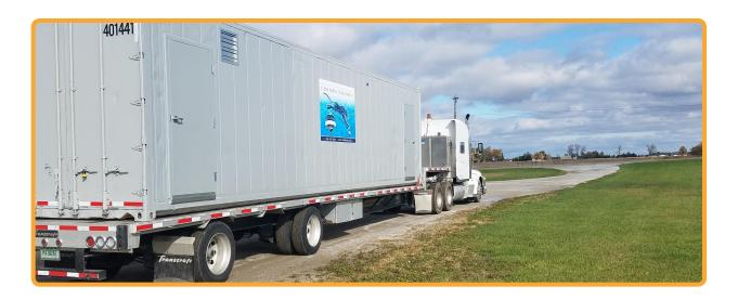
As a result of the success of the trial, IFM designed and constructed a modular treatment system to reduce ammonia. Built inside two 40' shipping containers, a 15,000 GPD UF/RO system was built and shipped to the site.
