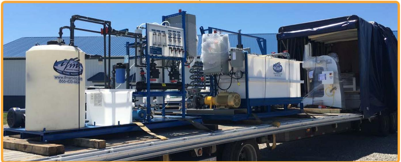
the use of an oil/water separator (OWS), ultrafiltration (UF) system, and was finished off by a reverse osmosis (R.O.) system in series. Each piece of equipment was individually skid-mounted and shipped down to its destination to be met and installed by IFM technicians.
