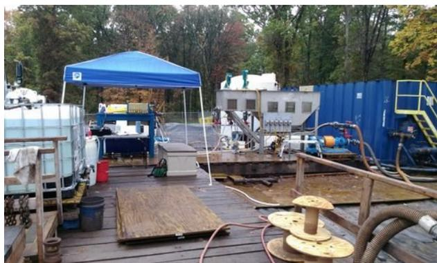
The horizontal clarifier is a perfect complement to ultrafiltration as the UF cannot tolerate the presence of free oil. IFM would recommend inline monitoring equipment to direct clarified water to the clean water treatment or to the UF System during times of floating solids, upset or other problems.
