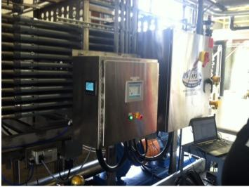
A major manufacturer of acrylic emulsions contracted with IFM to design and build a new upgraded, automatic ultrafiltration system. System enhancements were included in the design that upgraded in tank pumping design to ANSI pump with new improved seal design using seal plan 53A to combat fluid's tendency to congeal and cause short mechanical seal life. System designed with automatic CIP features, permeate recycle and advanced alarming and networking with site's DCS system for remove monitoring.
