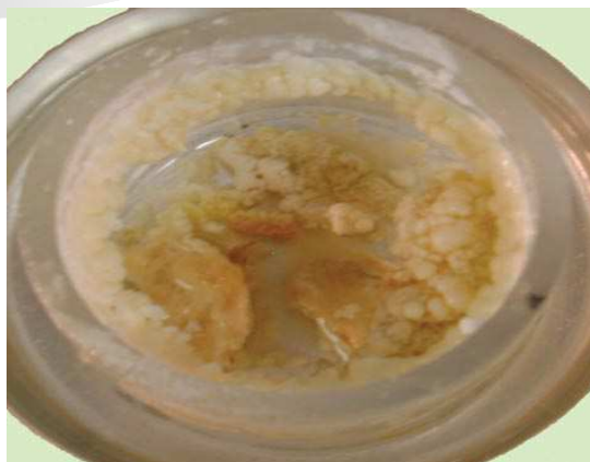
Figure 4. The photos illustrate a dramatic difference on grease treated with product containing BioS 3112. The control and non-BioS 3112-treated grease experienced 1.5% and 6.5% solids losses, respectively, while the BioS 3112 treated cells lost 42.9% of their solids.
